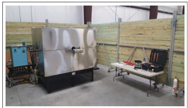
Performance Verification chamber -100f to +850f and API 6A Appendix F PR-2 Testing
